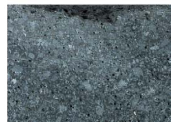
TufDura S600 Abrasion loss 4.0 cc.
