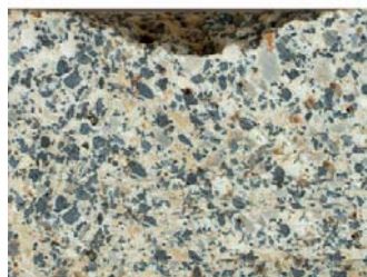
TufDura S300 Abrasion loss 5.0 cc.
